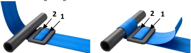
2. Make sure the strap end protrudes at least 100 mm [4"] or even longer from slot 2. If it is less than 100 mm [4"] disassemble and start over again. If longer, roll in the strap end and fix it by a cable tie to the shoulder belt.
